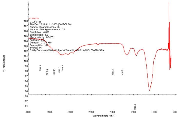
Figure 10. FTIR Spectra for Water-Soluble Contaminant from Fuel Filter #2
