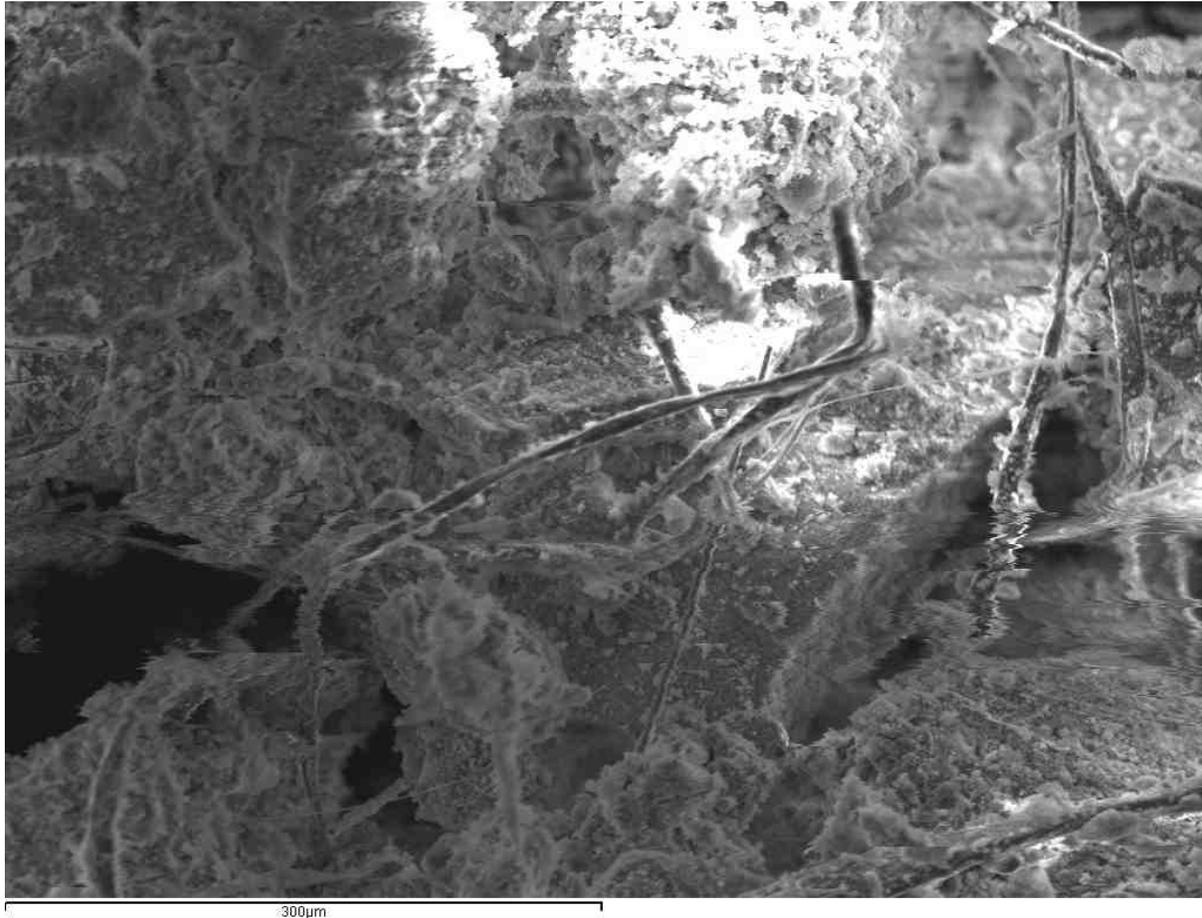
*Fig 14: Debris extracted from Fuel Filter*
