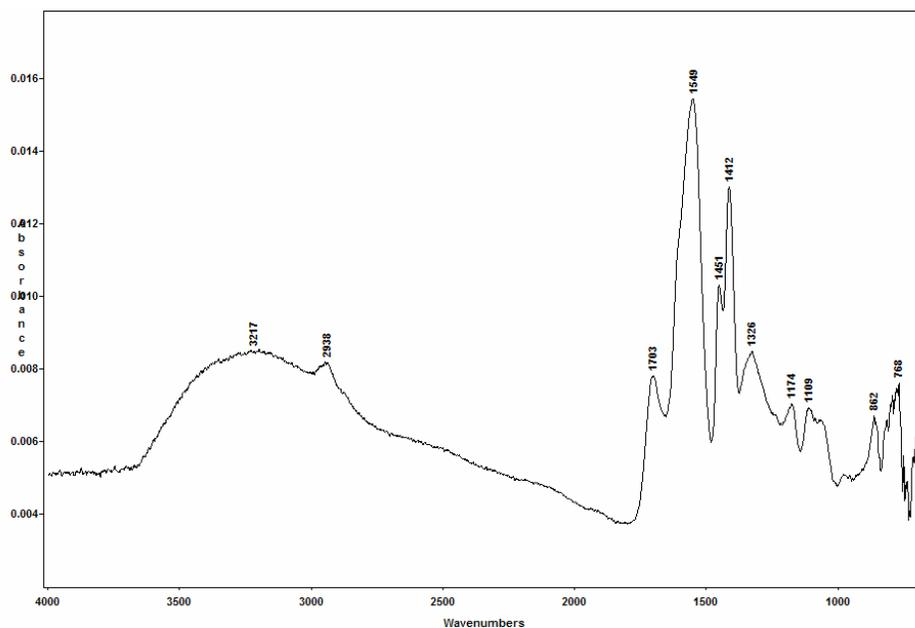
Figure 16: Reference FTIR of CuSO<sub>4</sub>/water treated Polyacrylate Polymer
