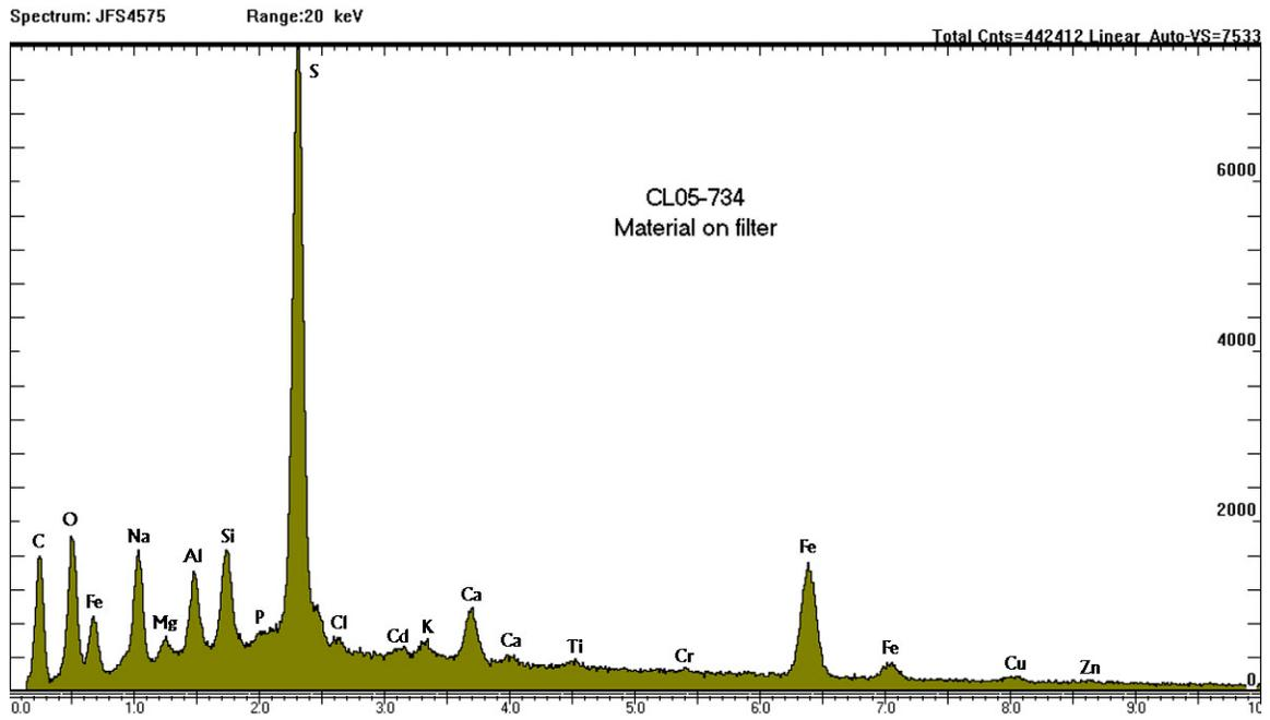
**A5. XRF of Fuel Filter #5 Contaminant**
