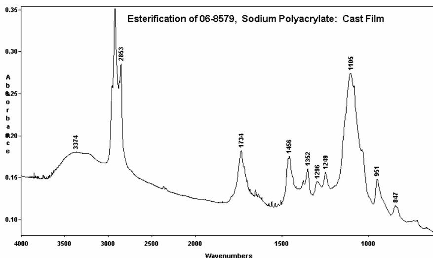
Figure 9: FTIR of Reference Sodium Polyacrylate after Esterification
