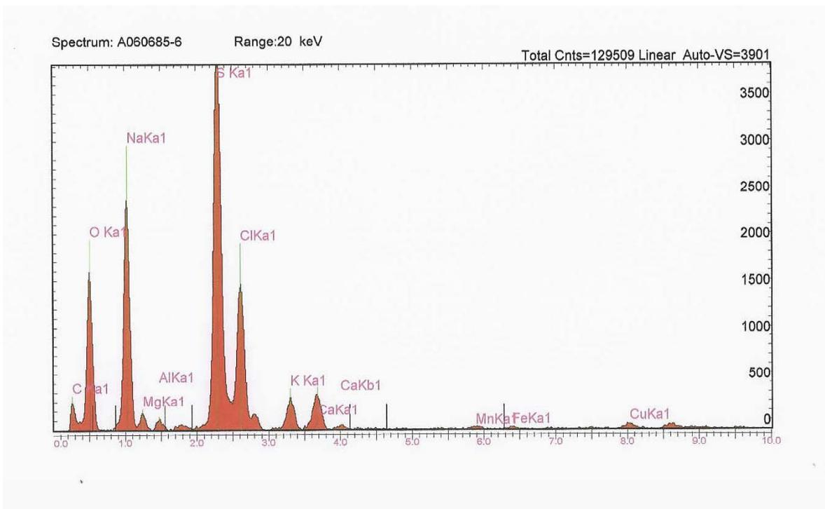
Figure A6. EDX spectrum of non-volatile residue from water extract of filter element B1.
