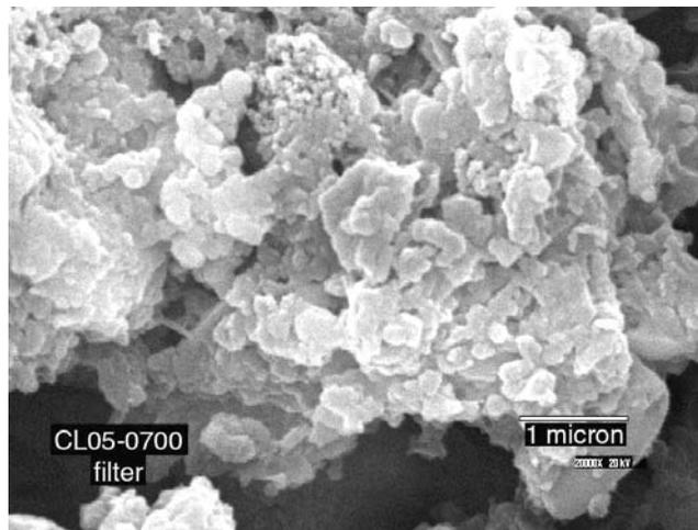
**Figure 6. SEM of Contaminant from Fuel Filter #4**
