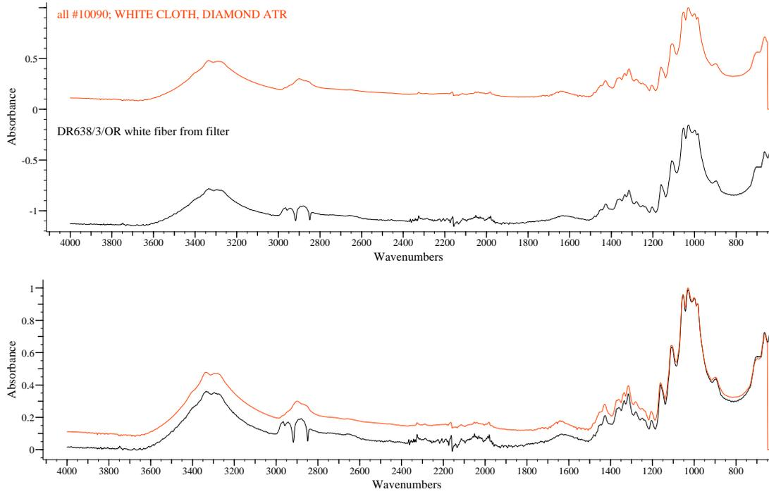
*Fig 9: IR spectrum of white fibers taken from filter folds compared with white cloth, spectra collected on diamond ATR*
