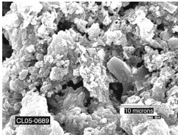
**Figure 3. SEM of Contaminants from Fuel Filter #3**
