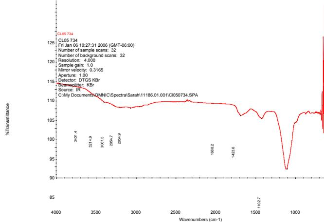
Figure 14. FTIR Spectra for Water-Soluble Contaminant from Fuel Filter #5
