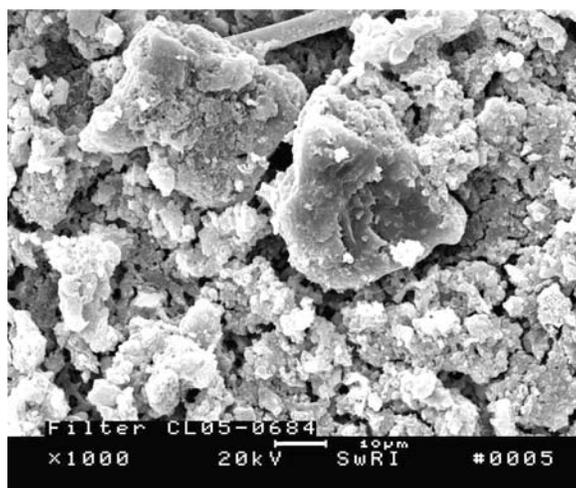
**Figure 4. SEM of Contaminants from Fuel Filter #2**
