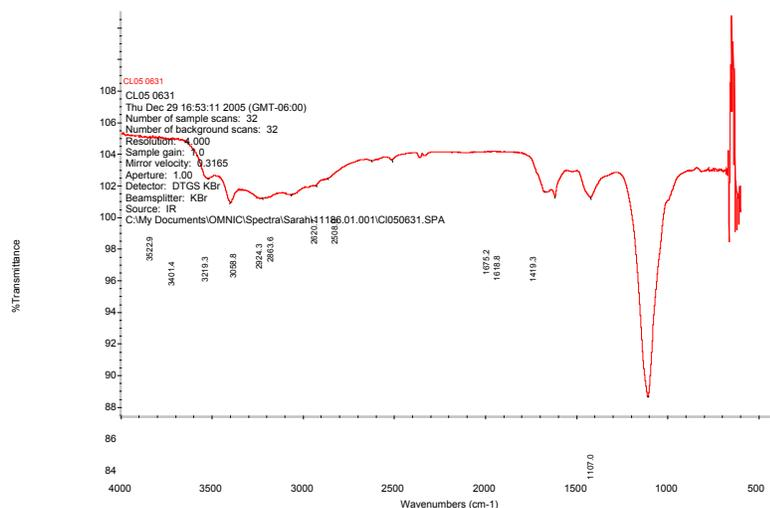
Figure 8. FTIR Spectra for Contaminant from Fuel Filter #1
