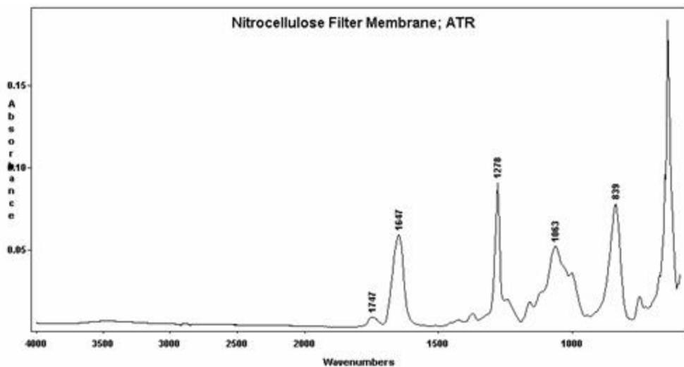
Figure 12: Reference FTIR of Nitrocellulose Filter
