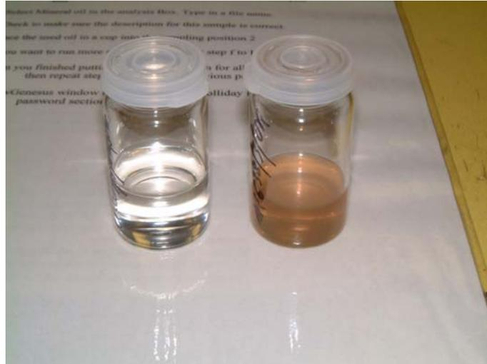
Fig 13: Fuel with suspended solids (right), Fuel after removal of solids by centrifugation (left)
