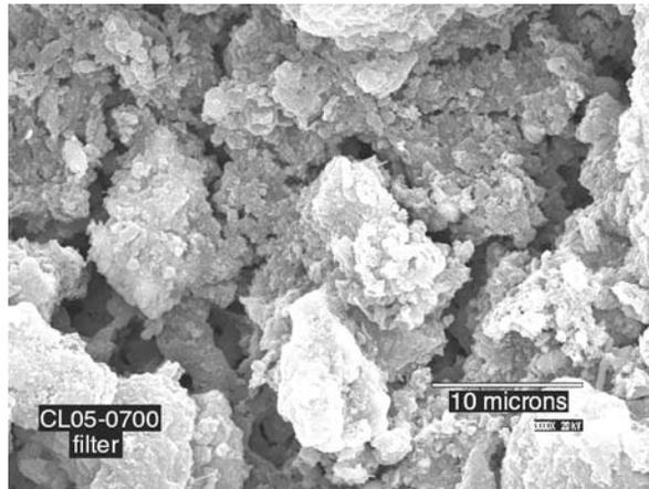
**Figure 2. SEM of Contaminants from Fuel Filter #5**
