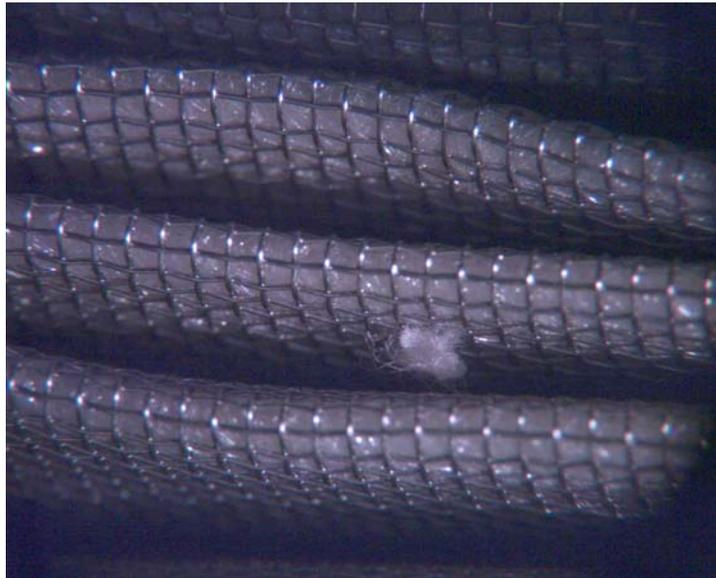
*Fig 8: White fibrous material in filter fold*
