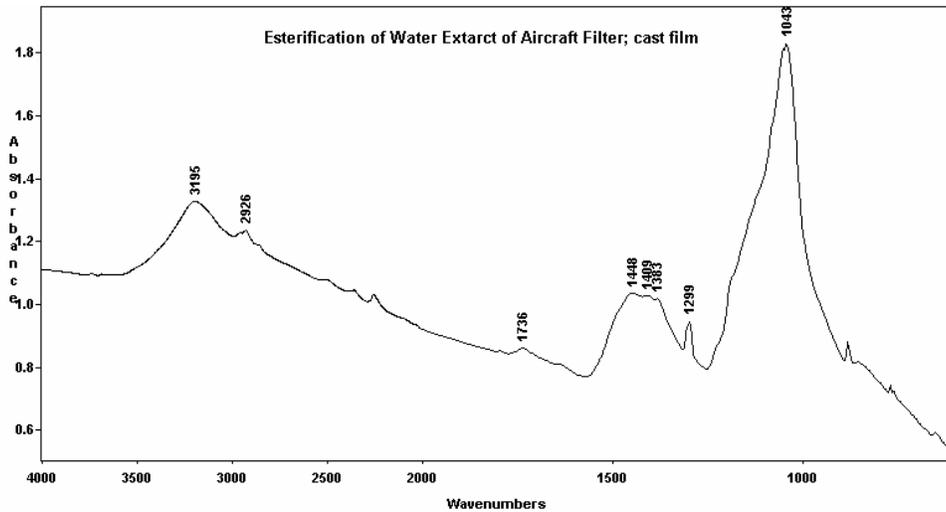
Figure 11: FTIR of Esterified Water Extract from Operator Q Filter 2
