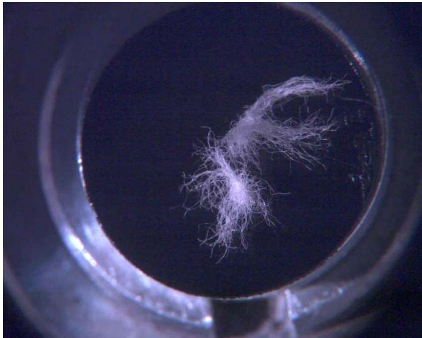
*Fig 10: Light microscope image of white fibers on SEM stub (Stub diameter = 140mm)*
