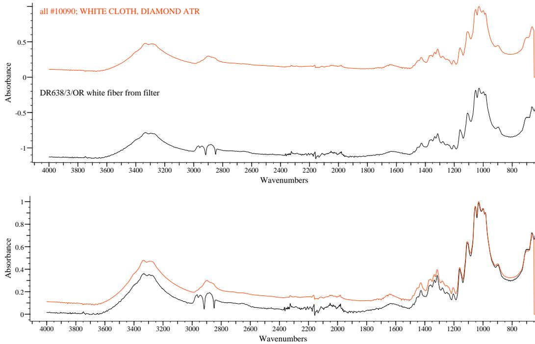
**Figure 8-17 IR spectrum of white fibers taken from filter folds compared with white cloth, spectra collected on diamond ATR**
