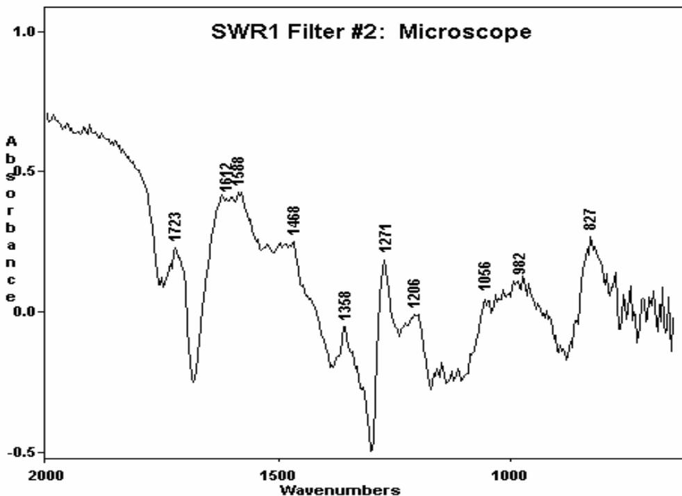
Figure 19: FTIR of Blue Particles from Debris after Isooctane Sonication
