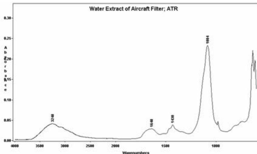
Figure 8: FTIR of Operator Q Filter 2 - Solid Removed After Water Sonication
