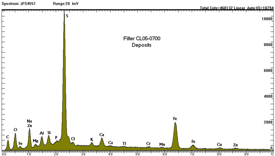
A4. XRF of Fuel Filter #4 Contaminant
