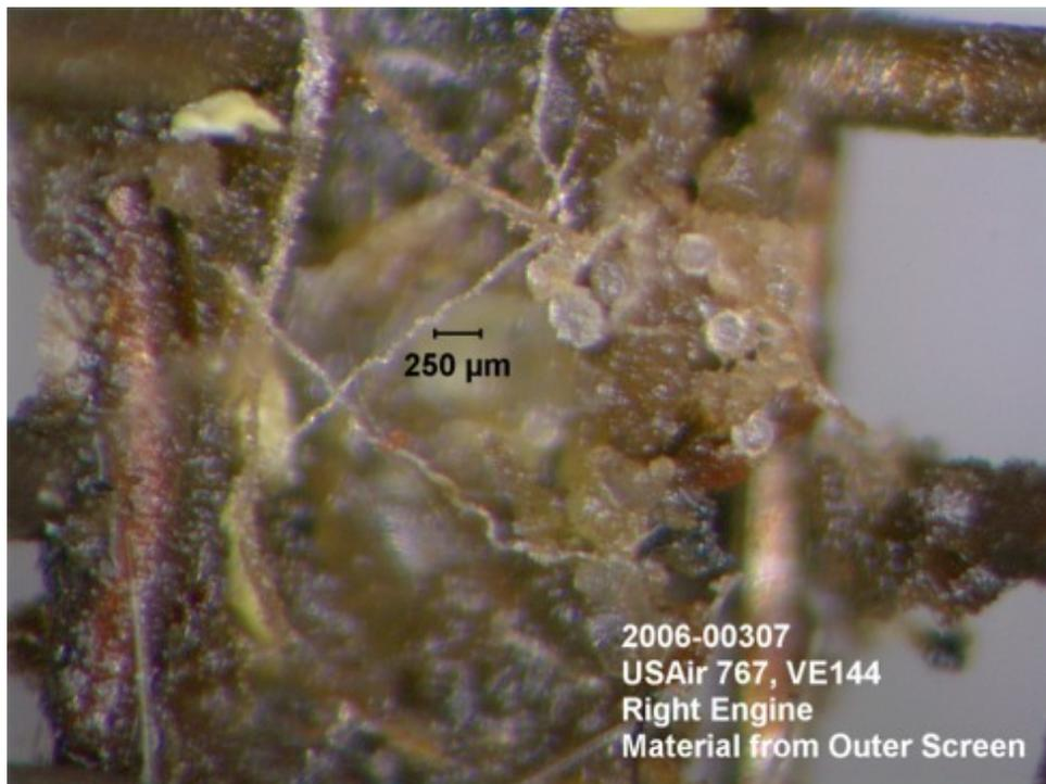
Fig.3 Filter's media clogged with clay, mineral particles and plastic-like beads
