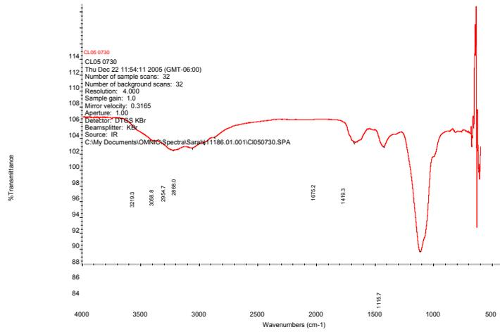
Figure 13. FTIR Spectra for Water-Soluble Contaminant from Fuel Filter #4
