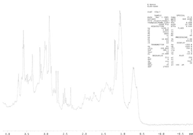
**Figure 17. NMR on Water-Soluble Contaminant from Fuel Filter #2**
