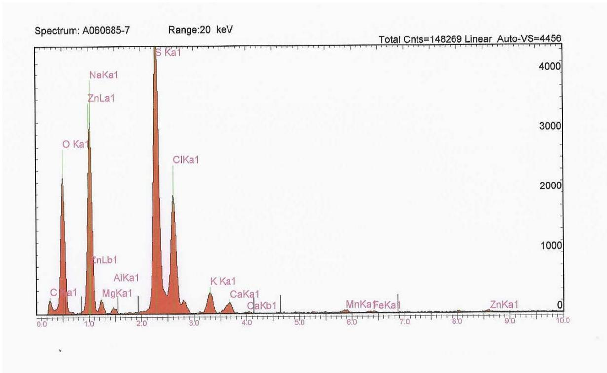
Figure A7. EDX spectrum of non-volatile residue from water extract of filter element D1.
