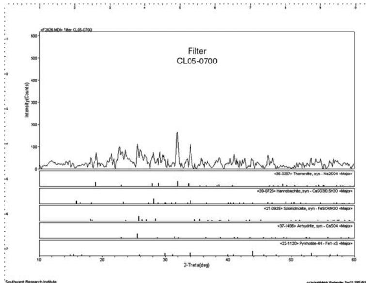
Figure 7. XRD Analysis of Contaminant from Fuel Filter #4
