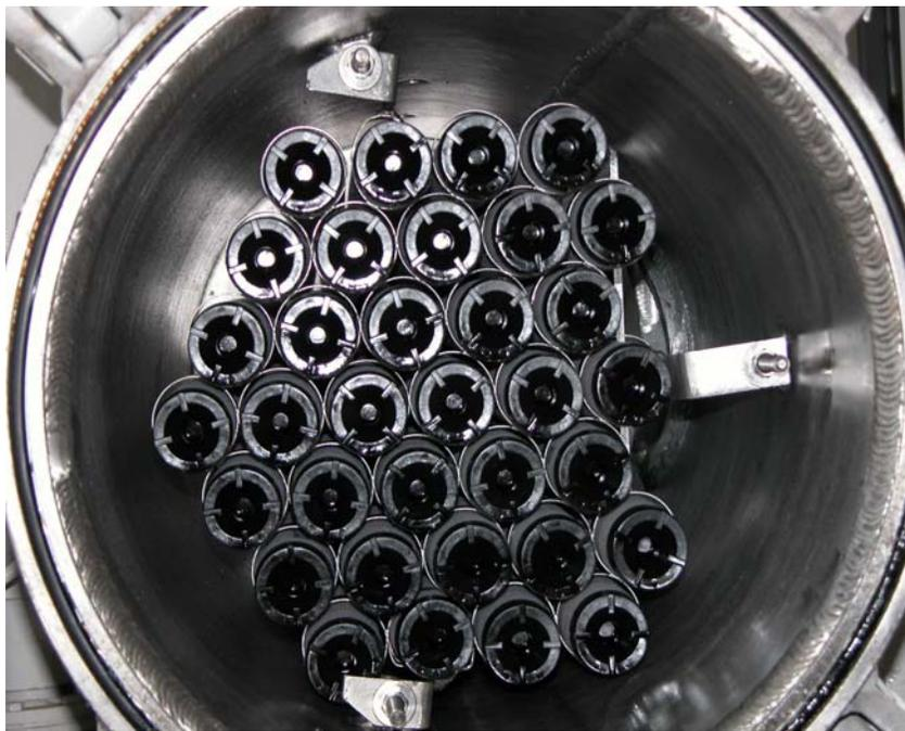
Figure 3-3 Inside View of Filter Monitor Vessel. Picture Courtesy ExxonMobil
