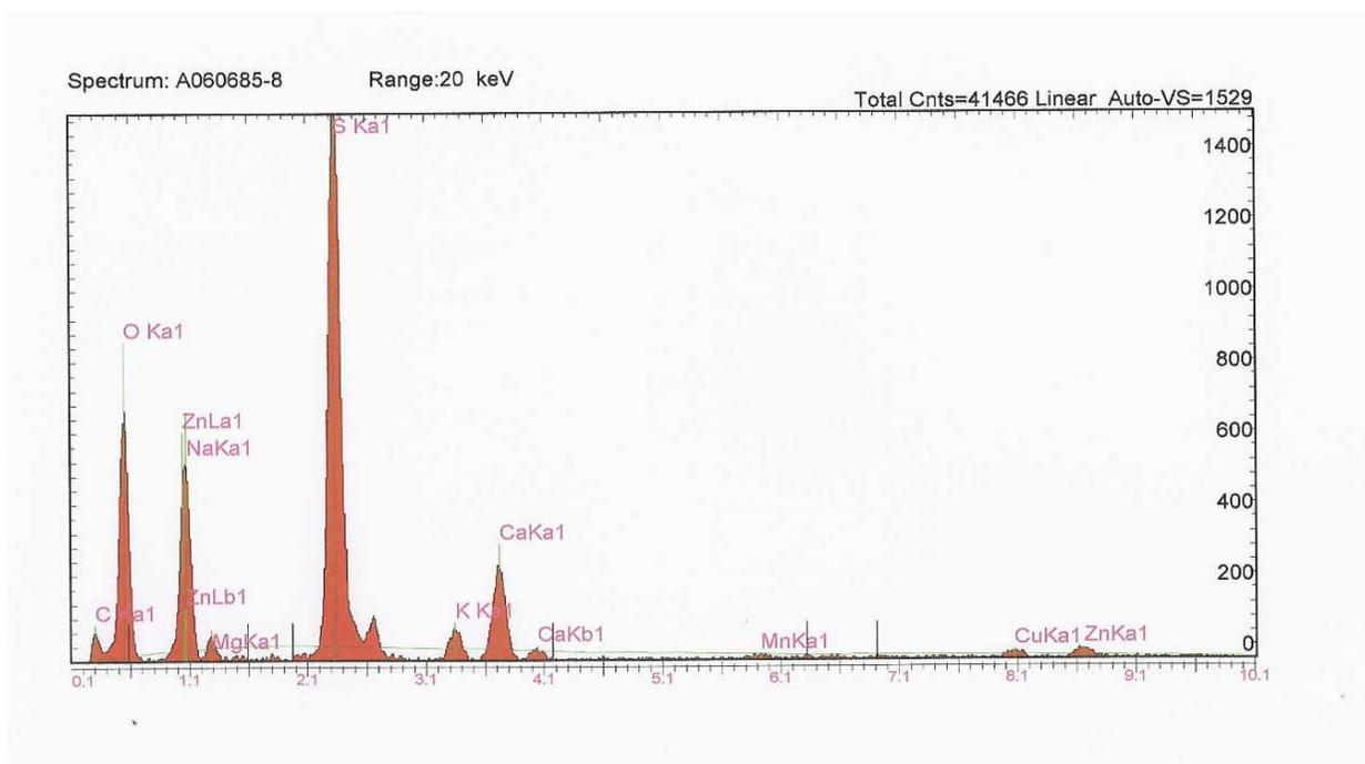
Figure A8. EDX spectrum of non-volatile residue from water extract of filter element H2.
