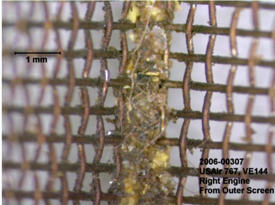
Fig.2 Upper mesh of the filter, plastic-like beads in the debris
