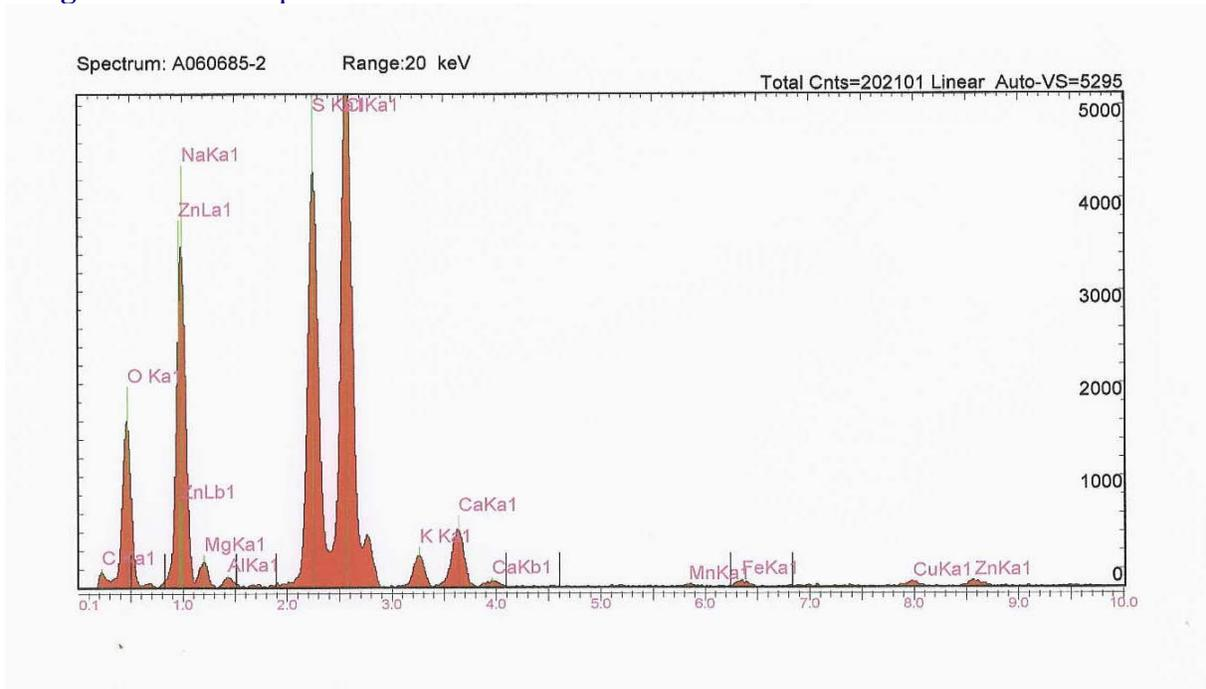
**Figure A2.** EDX spectrum of non-volatile residue from water extract of filter element G1.
