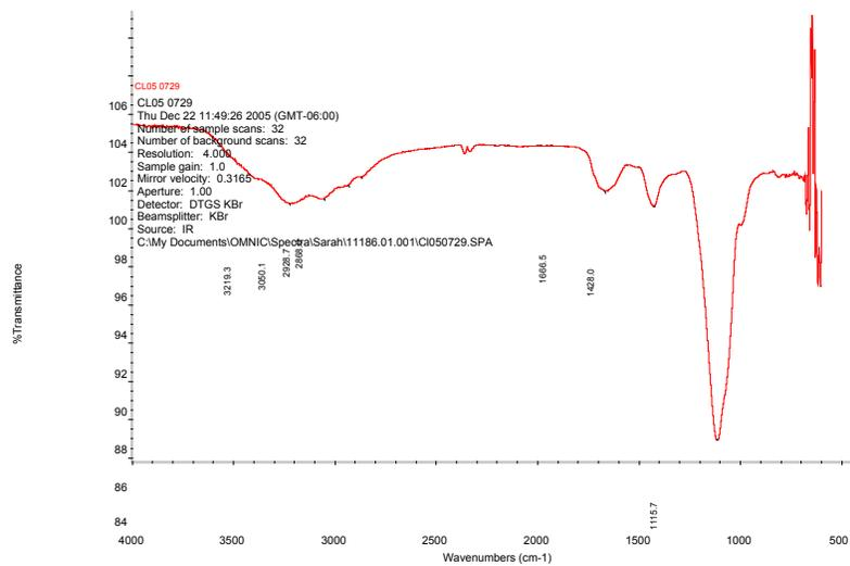
Figure 12. FTIR Spectra for Water-Soluble Contaminant from Fuel Filter #3
