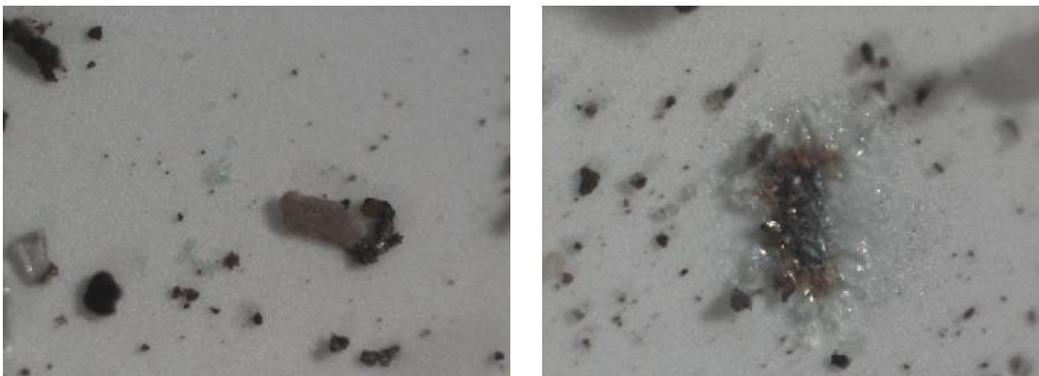
**Figure 8-14 Photomicrographs depicting blue copper sulphate – SAP adduct (attributed to SAP) in engine fuel filter elements F1 (Left) and G1 (Right)**
