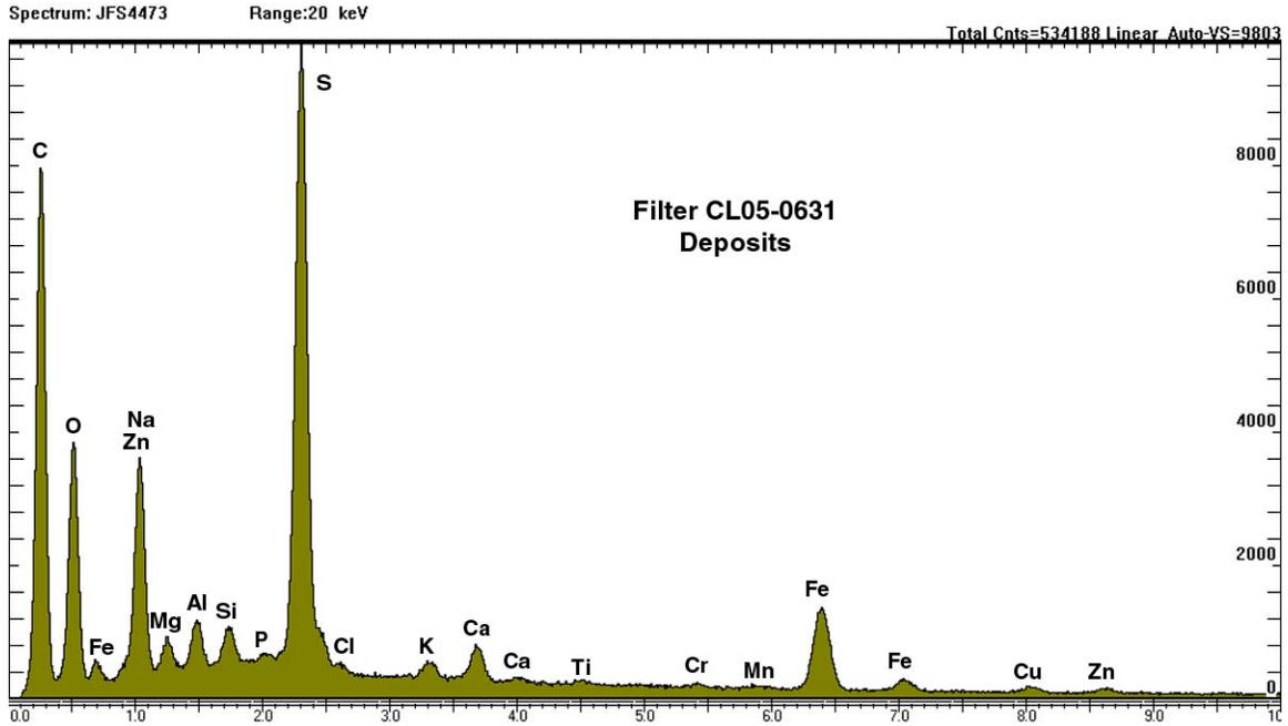
**A1. XRF of Fuel Filter #1 Contaminant**
