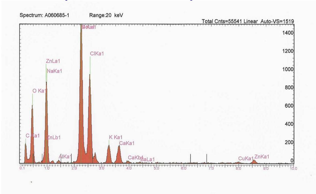
**Figure A1.** EDX spectrum of non-volatile residue from water extract of filter element F1.
