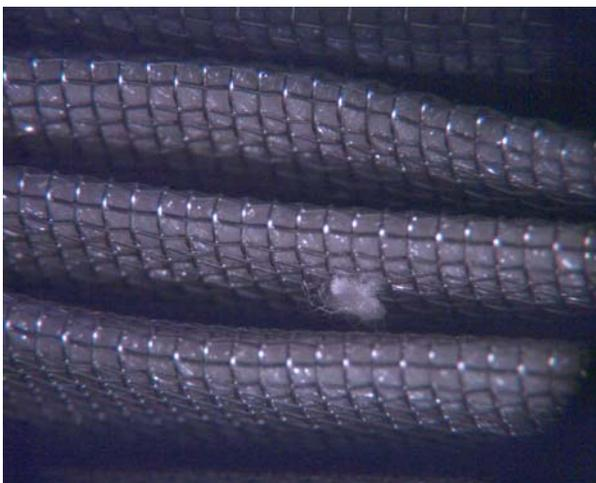
Figure 8-16 White fibrous material in filter fold
