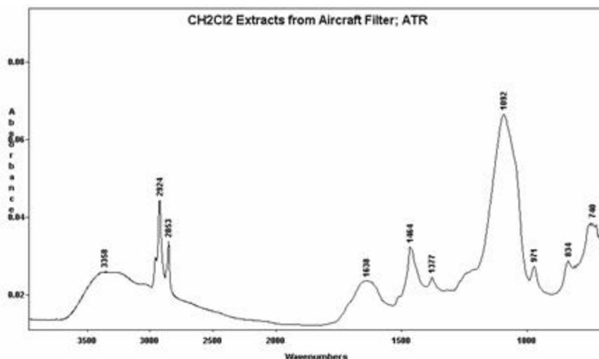
Figure 7: FTIR for Operator Q 1 Filter 2 - Solid Removed After  $\text{CHCl}_2$  Sonication
