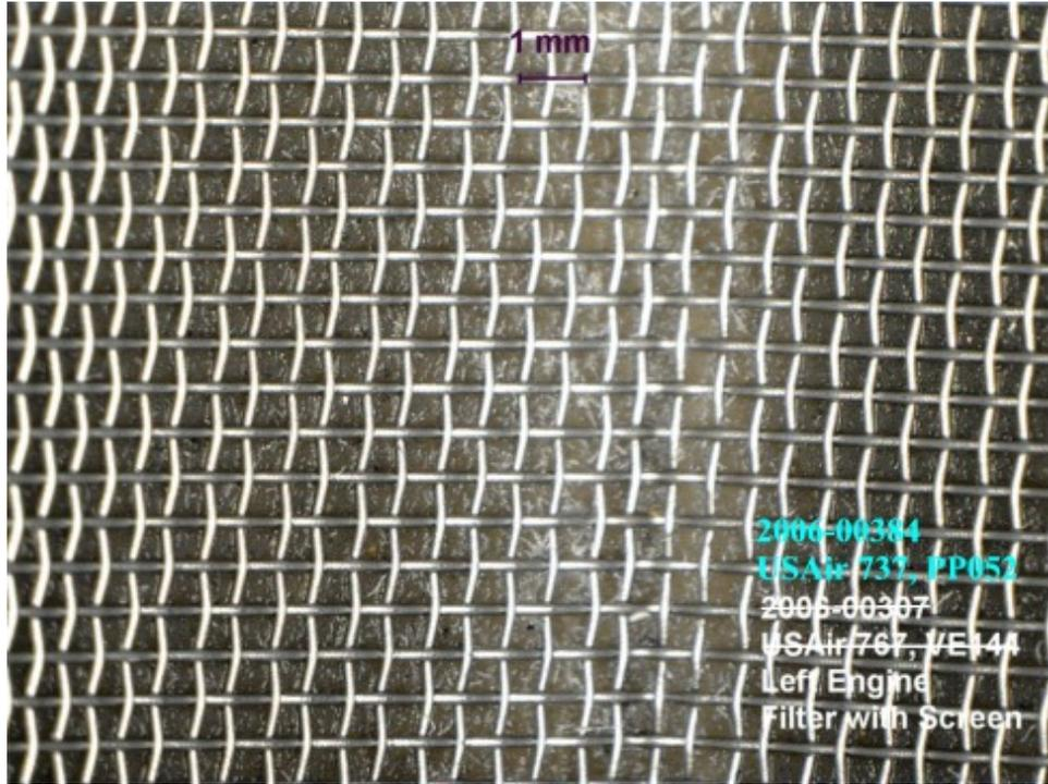
Fig.2 US Air 737 PP052 left engine fuel filter, filter's media
