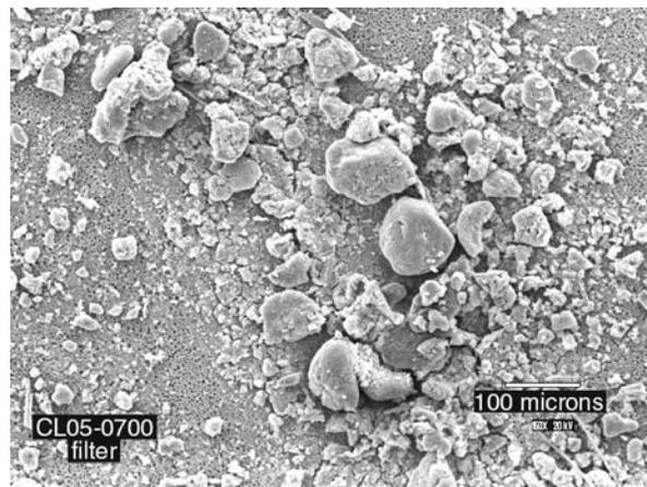
**Figure 1. SEM of Contaminants from Fuel Filter #5**
