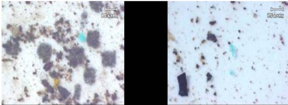
**Figure 8-13 Photomicrographs depicting blue copper sulphate-SAP adduct (attributed to SAP) in engine fuel filter elements D1 (Left) and E1 (Right)**
