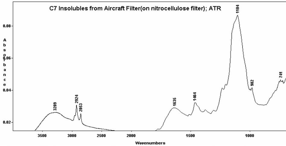
Figure 6: FTIR of Operator Q Filter 2 - Solid Remove After Heptane Sonication
