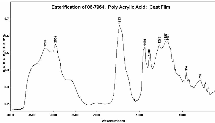
Figure 10: FTIR of Reference Polyacrylic Acid after Esterification
