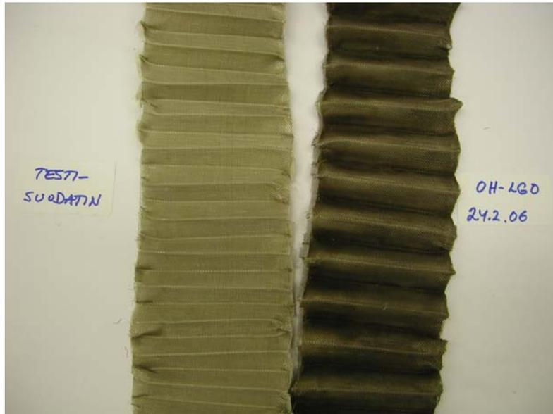
Photo 2. Filter mesh + paper filter
