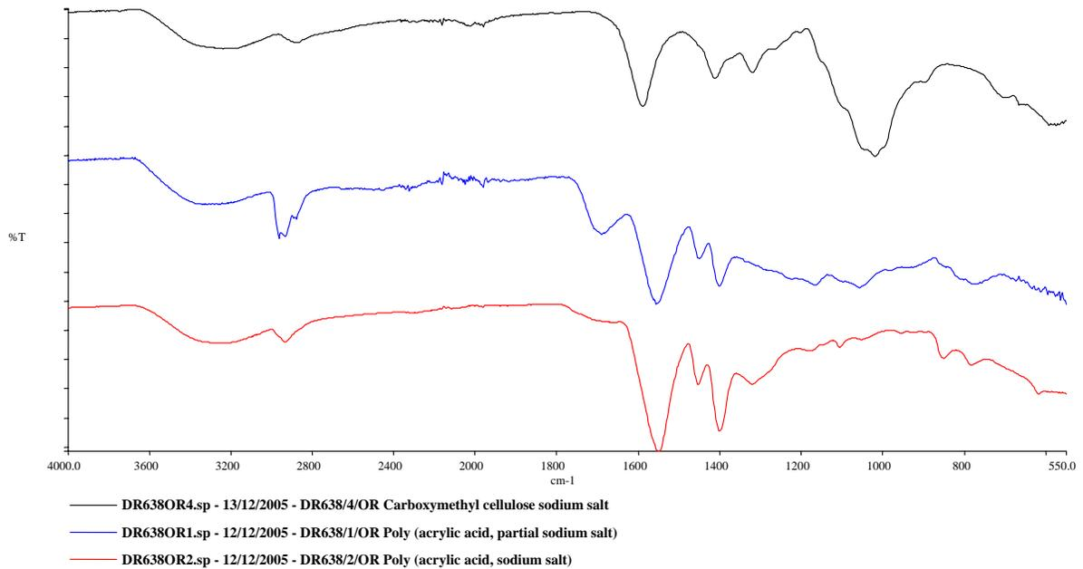
**Figure 8-22 IR spectra of reference SAP materials, collected on diamond ATR**
