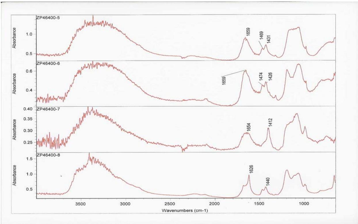
Figure 8-10 FT-IR Spectra of Non-volatile Residue Samples from the Water Extract.
