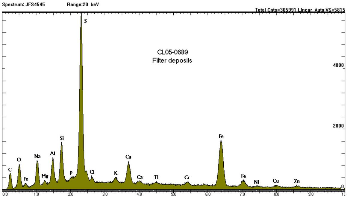
A3. XRF of Fuel Filter #3 Contaminant
