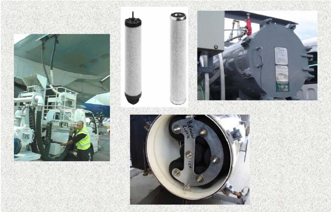
Figure 3-2 Water Absorbing Media Locations; Picture: Courtesy Continental Airlines
