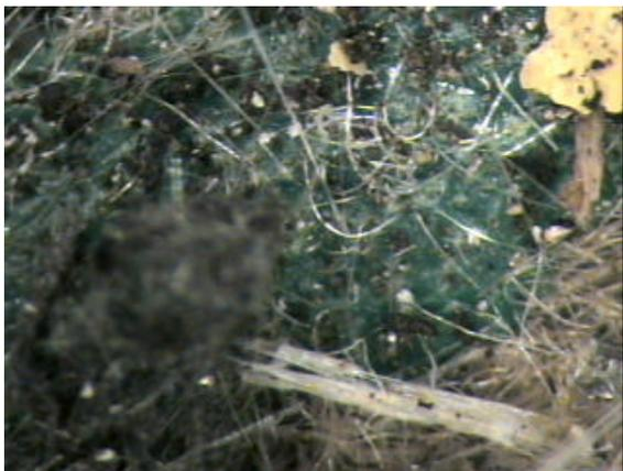
**Figure 1: Debris from Cut Filter**
