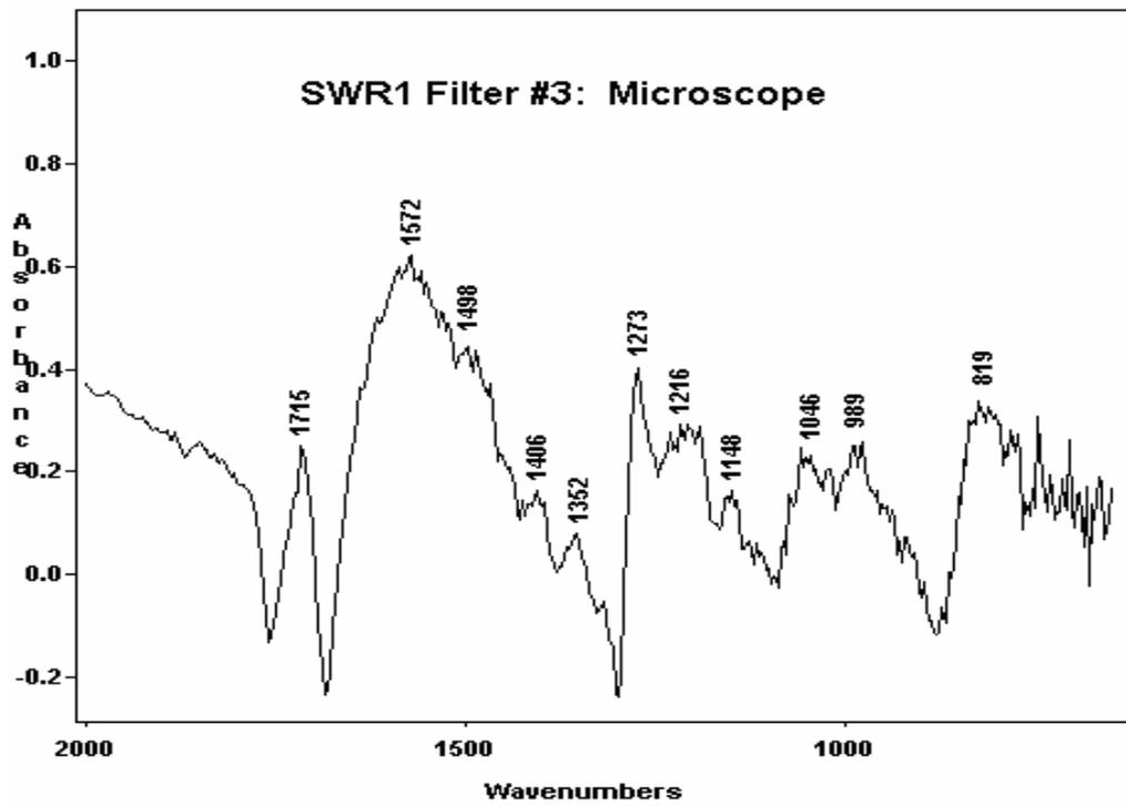
Figure 20: FTIR of Blue Particles from Debris after Water Sonication
