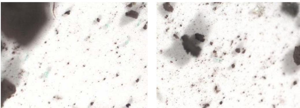
**Figure 8-15 Photomicrographs depicting blue copper sulphate-SAP adduct (attributed to SAP) in engine fuel filter elements H1 (both pictures)**
