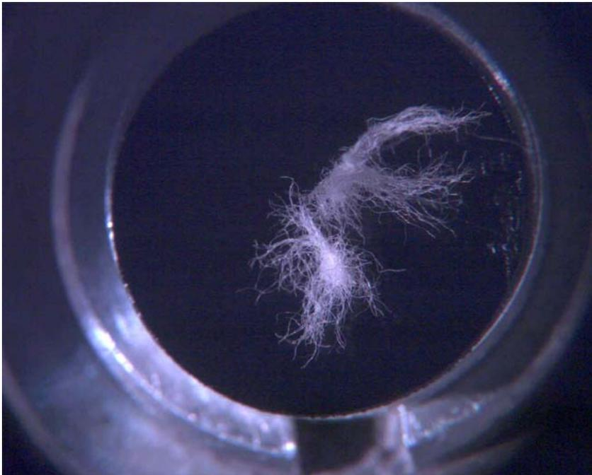
**Figure 8-18 Light microscope image of white fibres on SEM stub (Stub diameter = 140mm)**
