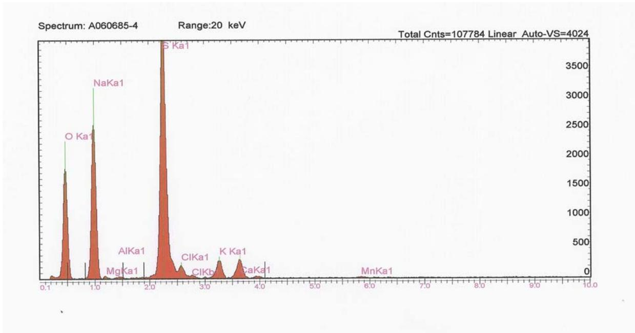
Figure A4. EDX spectrum of non-volatile residue from water extract of filter element A1.
