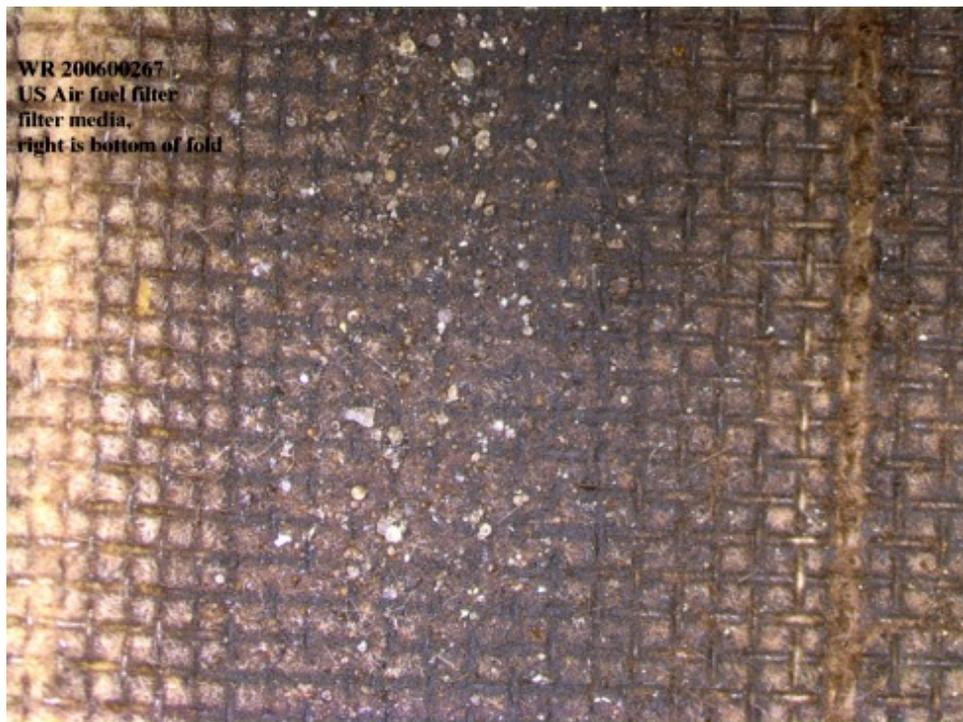
Fig.3 Clay deposits and plastic-like beads in the filter's media
