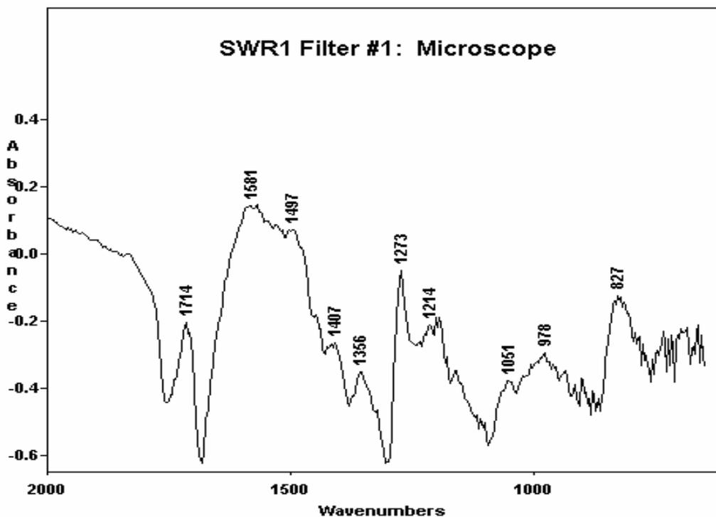
Figure 18: FTIR of Blue Particles from Loose Debris
