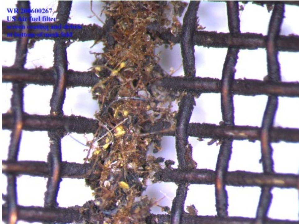
Fig.2 Filter's media clogged with clay, mineral particles and plastic-like beads
