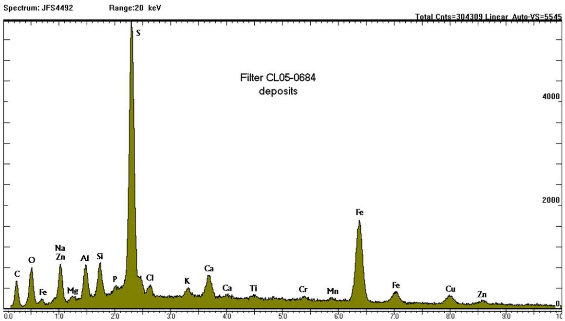
**A2. XRF of Fuel Filter #2 Contaminant**
