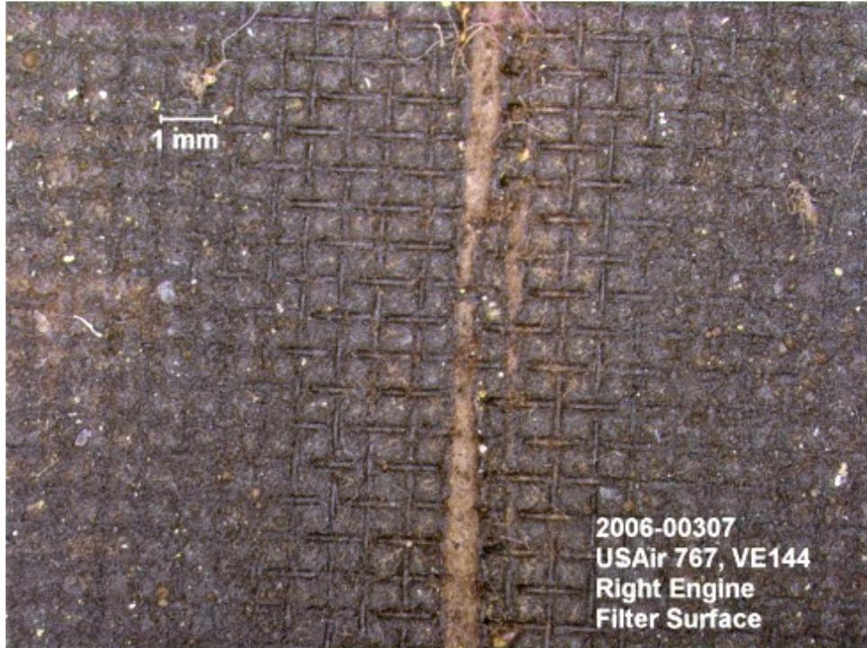
Fig.4 Clay deposits and plastic-like beads in the filter's media
