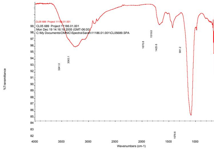
Figure 11. FTIR Spectra for Contaminant from Fuel Filter #3
