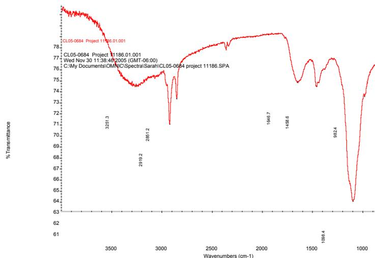
Figure 9. FTIR Spectra for Contaminant from Fuel Filter #2
