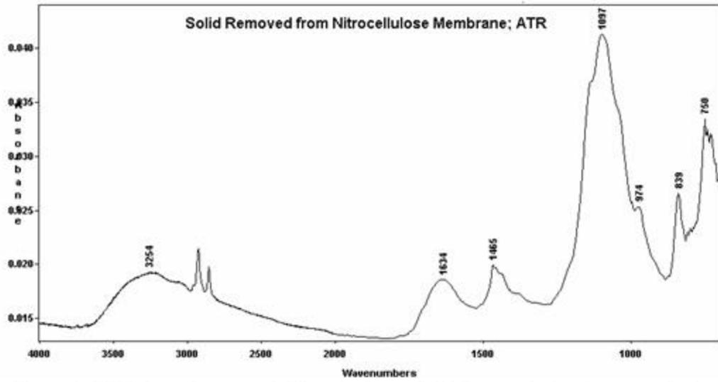
Figure 4: FTIR from Operator Q Filter 1 - Loose Solid Removed after Isooctane Sonication
