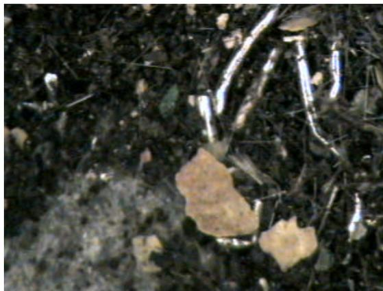
**Figure 2: Debris from Cut Filter**
