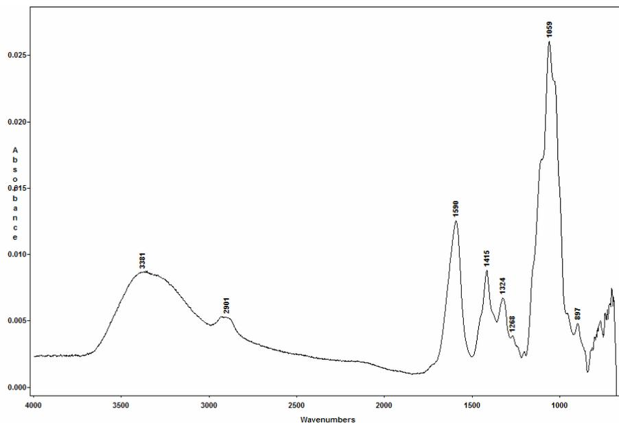
Figure 15: FTIR of Reference Carboxymethyl Cellulose after CuSO<sub>4</sub>/water Treatment
