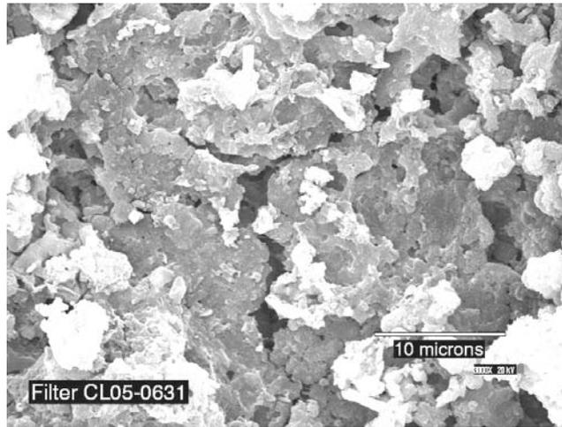
**Figure 5. SEM of Contaminants from Fuel Filter #1**
