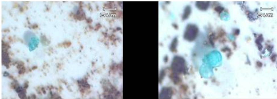
**Figure 8-12 Photomicrographs depicting blue copper sulphate-SAP adduct (attributed to SAP) in engine fuel filter elements B1 (Left) and C1 (Right)**
