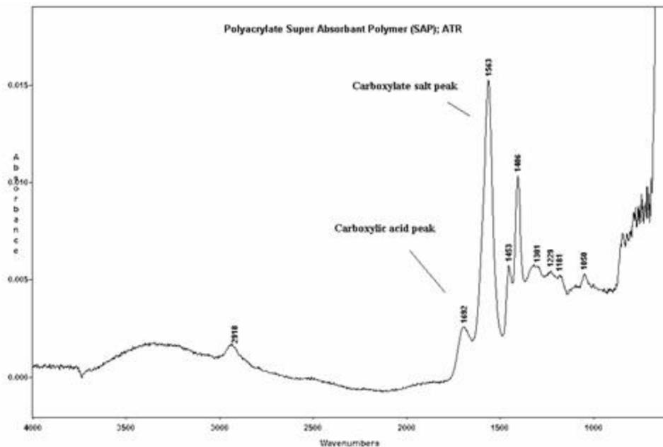
Figure 13: Reference FTIR of Polyacrylate
