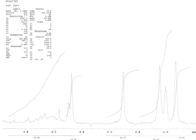
**Figure 16. NMR on Water-Soluble Contaminant from Fuel Filter #1**
