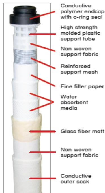
**Figure 3-1 2”diameter (Out to In flow format) Monitor Element – Electrostatically Conductive. Picture: Courtesy Racor/Faudi**
