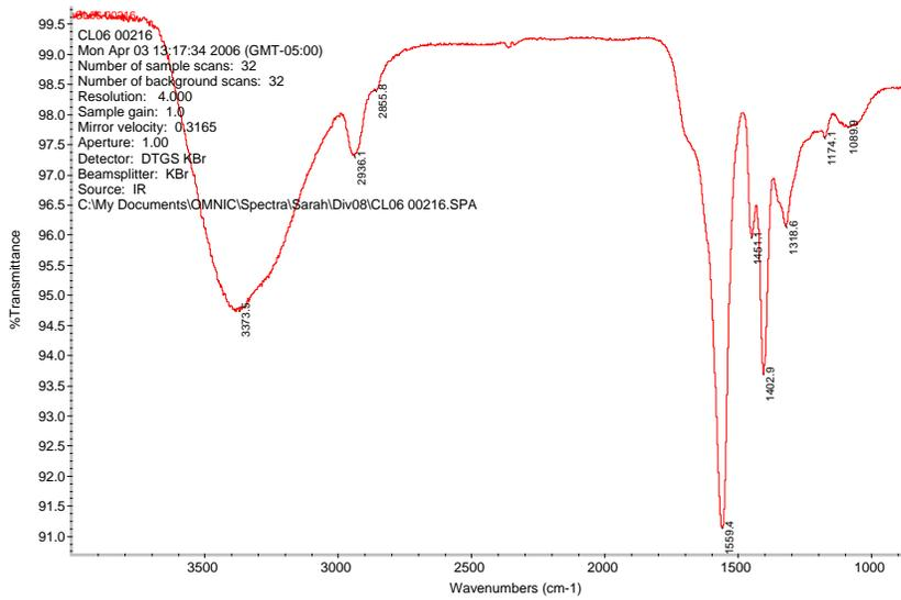
Figure 6. FTIR of water soluble contamination
