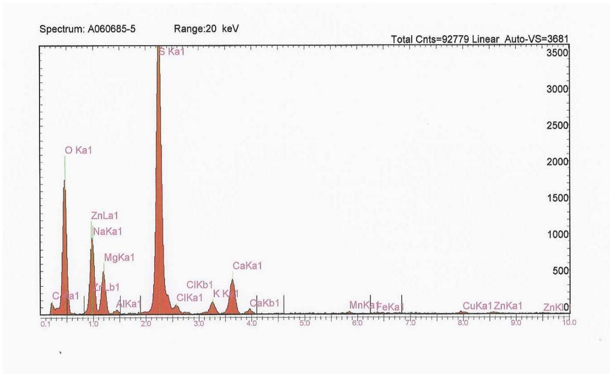
Figure A5. EDX spectrum of non-volatile residue from water extract of filter element C1.
