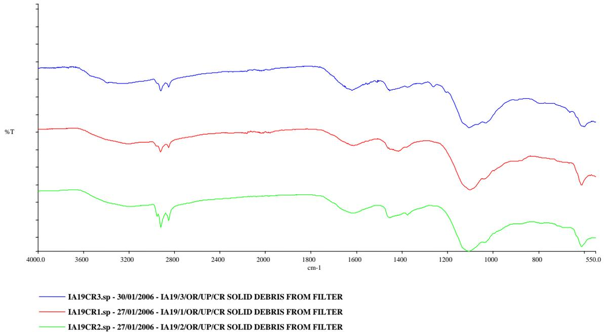
**Figure 8-21 IR spectra of solid debris from the three filters**
